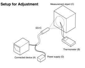
• Adjustment Example for the E5 N-L (Analog Input)
